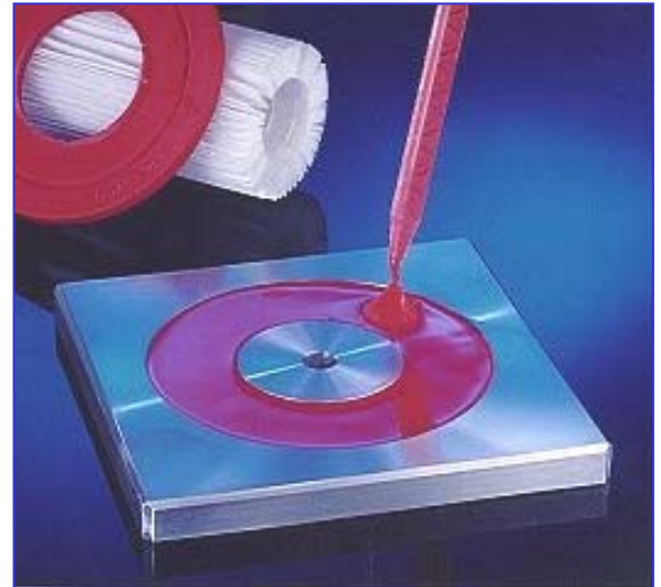
2-component polyurethane is applied into the end cap mold prior to inserting the filter element
