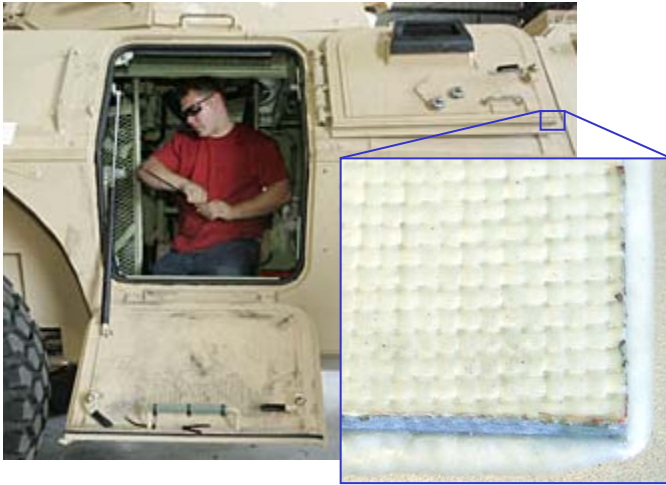
Kevlar Fabric is shown adhesive-bonded in position onto two door panel interiors
