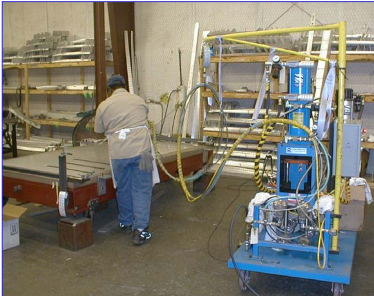
Applying Acrylic Adhesive to the Reflector Skin
