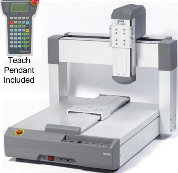
400 Series Bench Top XYZ Dispensing Robot 15.7" x 15.7" x 3.9" High Work Area
