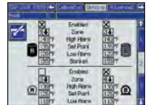
Set-up screen gives users easy access heat options
